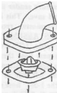
SJE Thermostat housing, Thermostat, & Gasket
