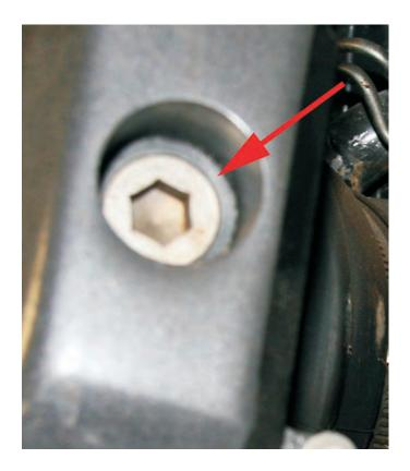
**Step 4.3:** We are now ready to install the hinge pins. Use the included Loctite on the threads and insert the hinge pin and Allen wrench into the hinge pin hole on either side. Be careful not to cross thread the hinge pin. Torque these to 80 Ft. Lbs.
