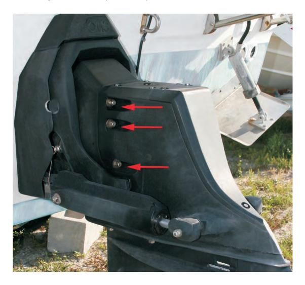
**Step 1.2:** Remove the six nuts and washers holding the upper unit to the bell housing. Once this hardware is removed the drive will be ready to remove. Simply pull back on the drive to remove it. If it is stuck you can tilt the unit up by hand and place a 2x4 between the drive and the transom assembly. Then let the drive rest on the 2x4. Now apply down pressure to the back of the drive to pop it loose.
