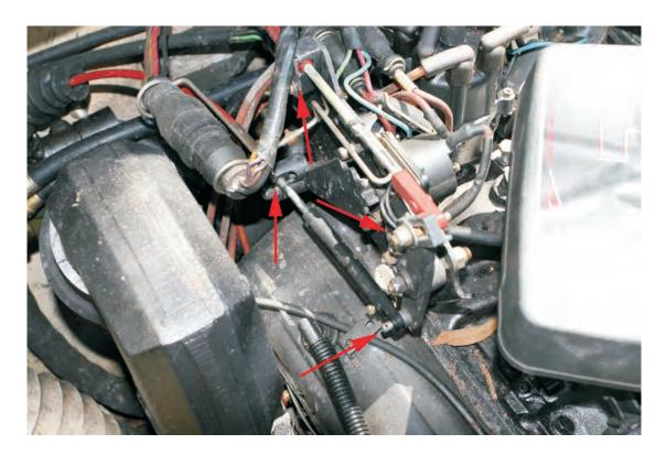
**Step 2.1:** To prepare the bell housing for removal. First we will go into the boat and disconnect both the intermediate cable (Bracket to Drive) and the remote control cable. We will remove the remote control cable at this point since it should be off when setting the shift adjustment. Remove any nuts or pins holding the cable on and then slide the cables off the pins. Retain the hardware for reassembly.
