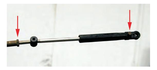
**Step 2.3:** Disassemble the cable end from the intermediate cable. Remove the small set screws and the cable end should slide off. Then loosen the jam nut and unscrew the barrel. Then the shift cable bellows can be removed.
