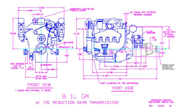
NOTE: This drawing is intended as a visual guide to the layout of this engine. The dimensions provided are intended for location and overall size.
